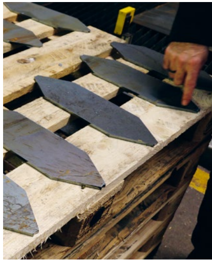
Left: Component for pipe supports
